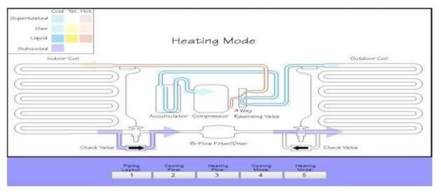
FIGURE 2 PIPING LAYOUT OF REVERSE CYCLE AIR CONDITIONER SYSTEM
